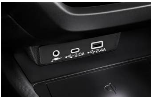
Front USB Ports (Type-A and C) and Rear USB Power Ports
